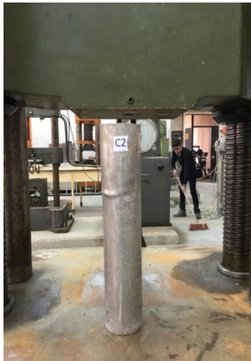
Figure 13. C2 , t=2\text{mm} (mode failure)
