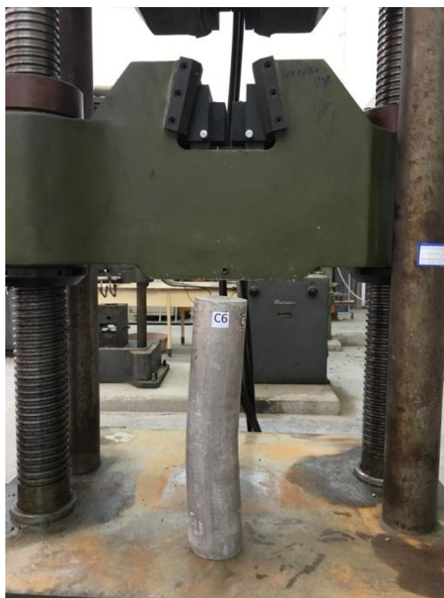
Figure 16. C6 ,t=5mm (mode failure)
