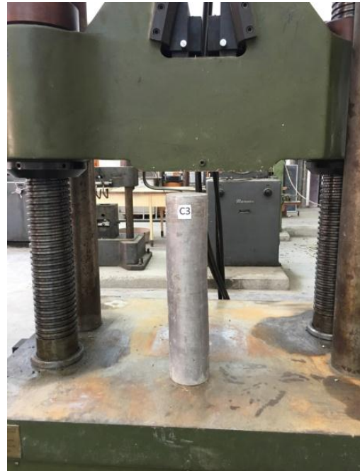
Figure 9. Reference column CR ,t=0mm (mode failure) Figure 10. C3 ,t=3mm (mode failure)
