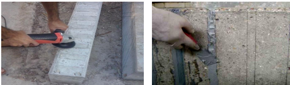
Figure 4. Roughing concrete surface and applying epoxy at CFRP strips location of a typical tested beam.
