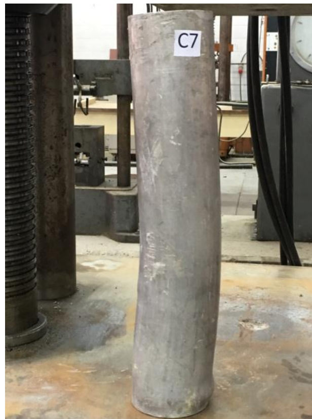
Figure 14. C7 , t=5mm with length 700mm (mode failure)
